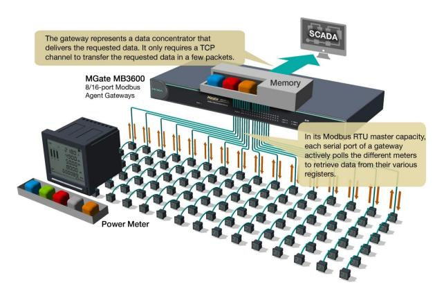
For any system integrator, easy configuration is always a high priority. In agent mode, the gateway in its RTU master capacity can set many Modbus commands. In order to save time with configuration, some gateway brands support comma-separated value (CSV) files, which can be easily configured and imported into the gateway by using excel.
