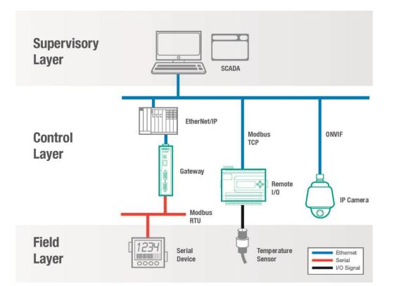
To meet industrial environment requirements, different transmission media can be used to build the most reliable communications system. For example, fiber-optic cable is used for Modbus RTU communications because it can extend over a long distance. In cases of excessive
