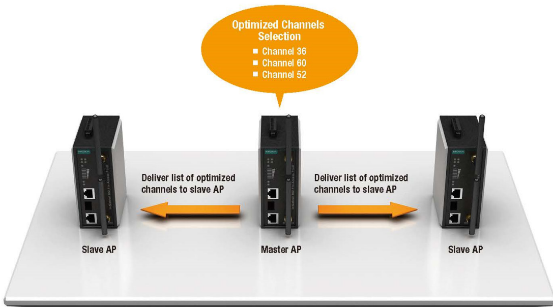
Figure 2: Master AP provides a list of the optimum channels to the Slave APs
