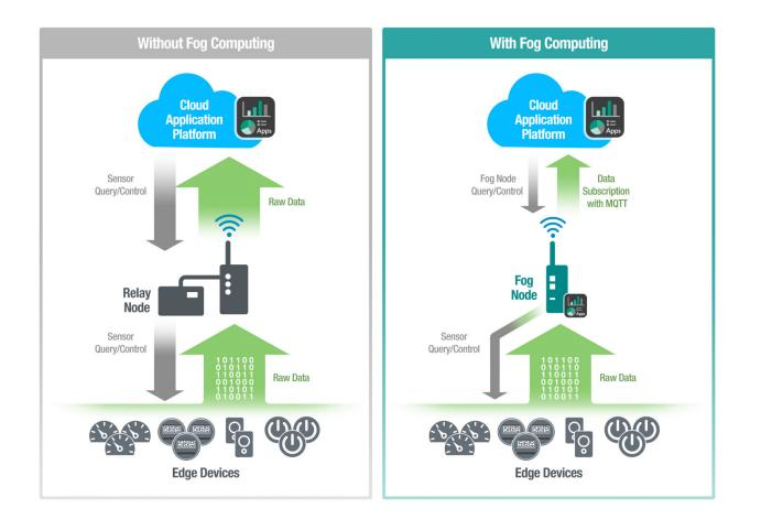
Fog computing works best in IoT-based systems with geographically dispersed end devices, where connectivity to cloud-based systems is irregular but low latency is a key requirement. IoT applications that periodically generate data in the order of terabytes, where sending data to the cloud and back is not feasible, are also good candidates for the fog computing model.
