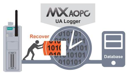
When the network fails and then recovers, the logger automatically retrieves data logs, with timestamp matching the duration of the disconnection, from the data buffers of specific ioLogik 2500 devices, and then pushes the supplementary data into the database.
