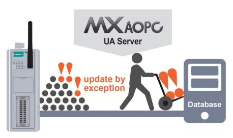
with big data, particularly since by its very nature, polling results in the collection of tons of worthless data from thousands of sensors, leading to high data storage costs and time consuming data analyses. When your sensors spit out data at a frequency much smaller than the polling interval, such as is the case when monitoring a machine's ON/OFF status, "updating by exception" can reduce the amount of data storage and increase the efficiency of data analysis.
